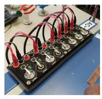
Prototypes of "coin cell" batteries that integrate the polymer binder technology are tested in Dr. Yu Zhu's lab
